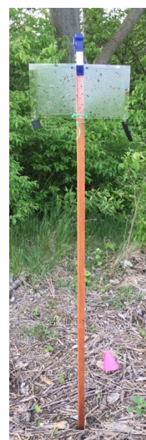
Figure 4. Sticky panel trap used to monitor stink bugs.
